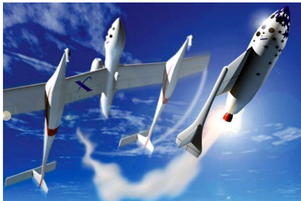
An artist's drawing shows SpaceShipOne 's rocket engine igniting seconds after release from its mothership, WhiteKnight .
